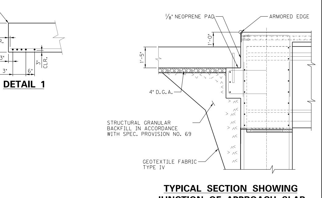
JUNCTION OF APPROACH SLAB WITH BRIDGE BACKWALL
