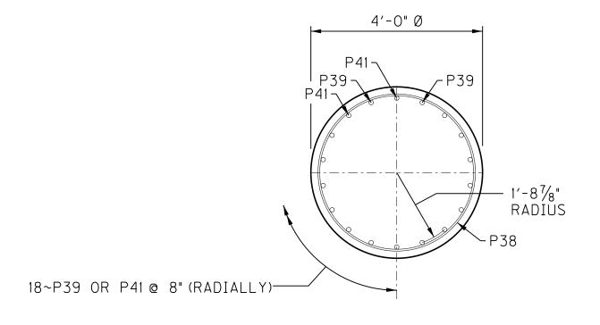
NOTE: USE A MECHANICAL COUPLER TO SPLICE P37 DOWEL TO P39 BAR AND P40 DOWEL TO P41 BAR, LAP SPLICES SHALL NOT BE USED.
